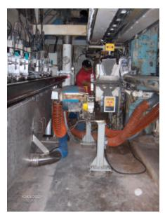
HSB carried out the engineering and design for system modifications on a machine. tissue Modifications included reconfiguring the sheet run, modifying the tail threading system, adjusting the dust extraction. assistance with the installation of state of the art water jet slitters, scanner relocation and a completely new trim handling system depositing the trim to three different pulpers.
